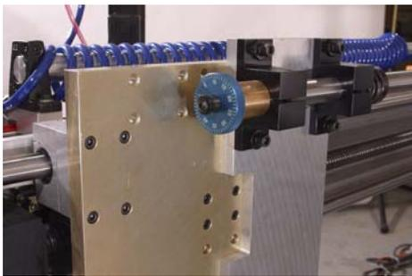
Rugged 1 1/8" dual ball screws and (4) 3/4" shafts handle the sheet movement. A 1000 watt closed loop D.C. servo motor/amplifier drives the system with speed and precision. Travel is 50"
