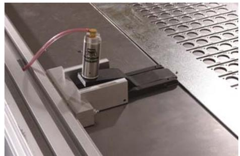
Side-to-side adjustable pneumatic fingers grip the workpiece for feeding. Grippers can be placed up to 8 ft. apart and travel up to 50" front to rear. Grippers can move to within 1" of the punch or shear blade. 1/8" dia. Pins on each gripper fit into a corresponding hole on the blank for accurate referencing.
