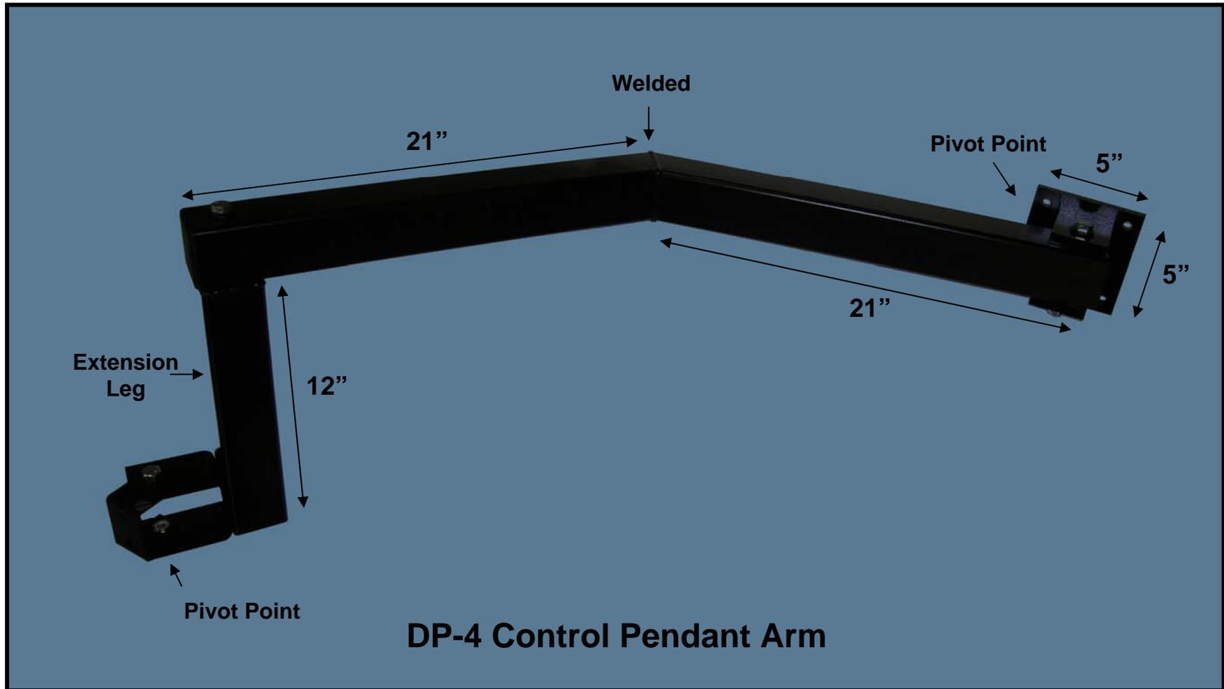
The DP-4 pendant arm can be bolted directly to all Automec controls. It is fabricated from 2 1/2" x 2 1/2" x 1/8" square steel tube.
